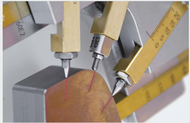
SKM 2: Measuring the wear of the running edge at three reference points
