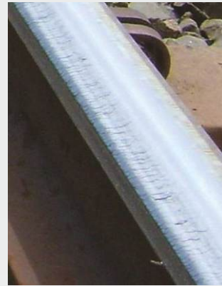
RCF on the rail surface and its mapping in the software
