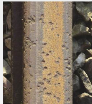
Pitting on the rail surface and its mapping in the software
