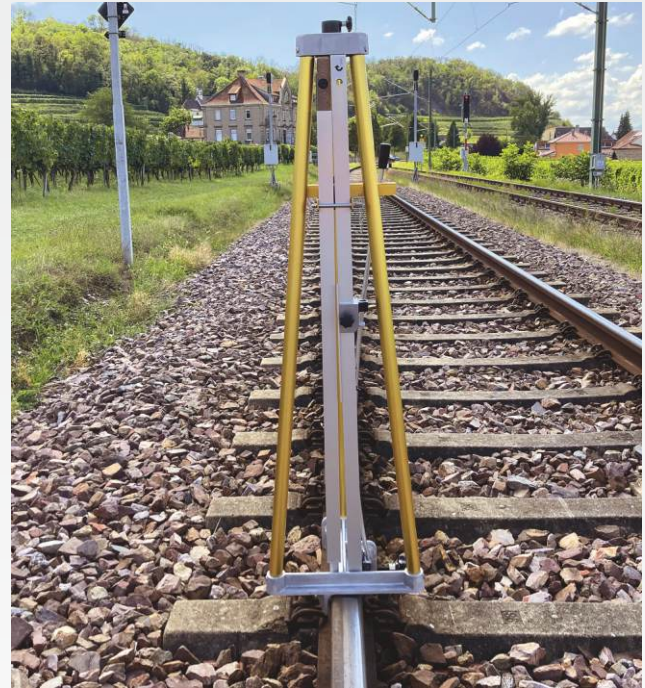
VIG 1300 with fixed and divided levelling stick
