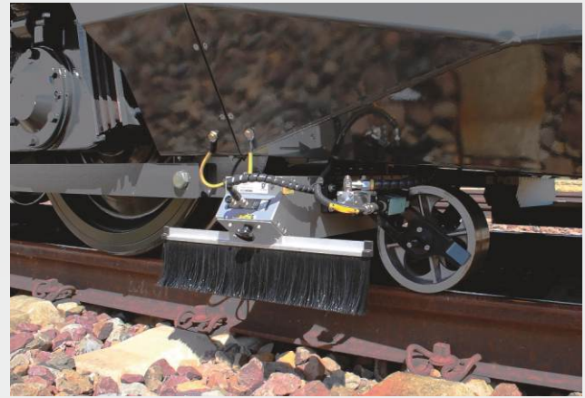
Integrated laser-based transverse profile measuring system
